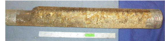
Corroded tube w/ammonia bisulfates on it
